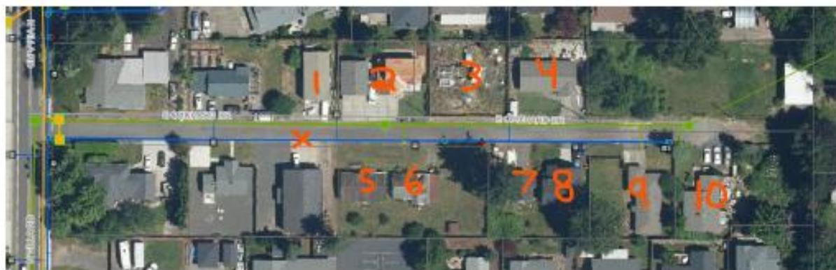
According to the City of Newberg Public Utility GIS, the "X" on the image above depicts where the 8" DI water main reduces down to a 4" DI water main. The calculations below assume up to 20 homes would be supplied by the existing 4" water main.
